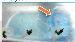
Example of the wave while shaking (4 L, 25 rpm). This kind of wave results in a good mixing time.
