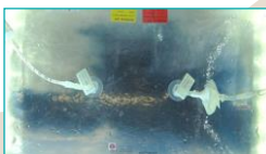
Example of the discolouration and a good parameter for the mixing time (4L, 25 rpm)
