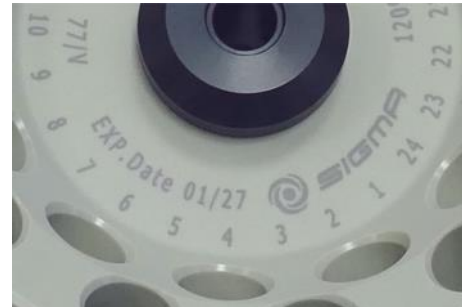
Fig. 8: Different service life – engraving on the bucket/rotor
