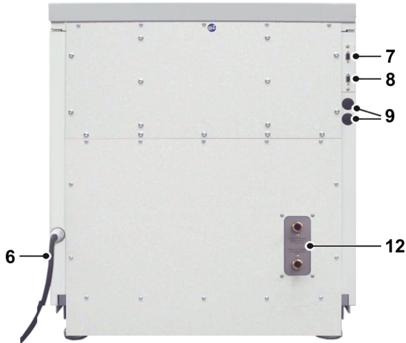
Fig. 5: Rear view of a water cooled centrifuge
