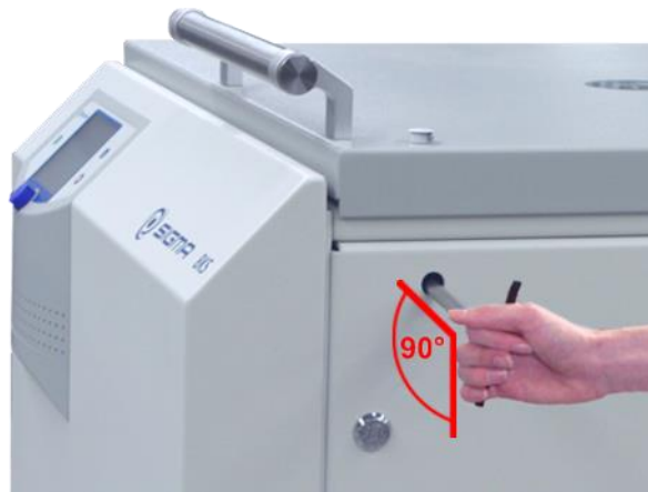
Fig. 48: The emergency lid release key must be inserted horizontally.
