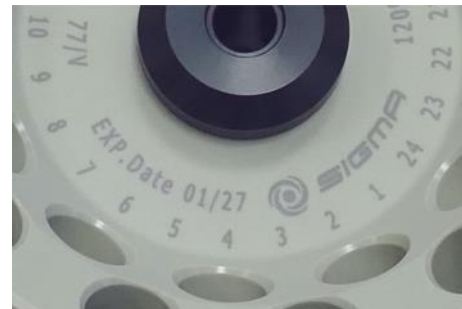
Fig. 4: Different service life – engraving on the bucket/rotor
