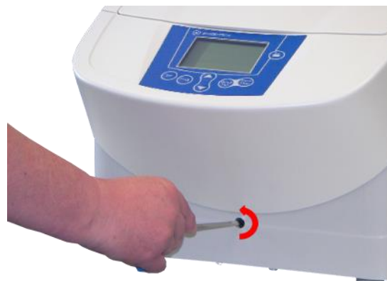
Fig. 9: Manual release of the lid lock
