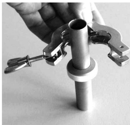
Fig. 56: Attaching the clamping ring
