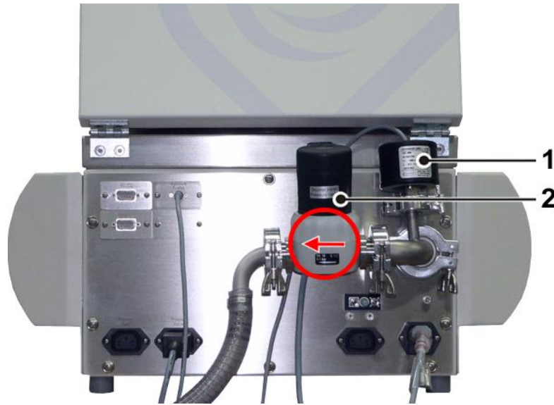
Fig. 8: Installation of the pressure control valve and the vacuum sensor
