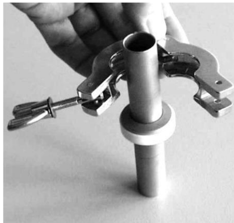
Fig. 51: Attaching the clamping ring
