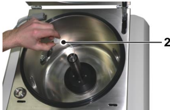
Fig. 57: Removing the electronic temperature measurement system
