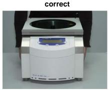
Fig. 6: Lifting the RVC
