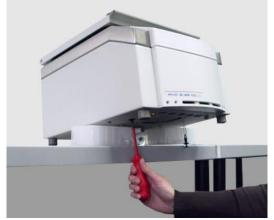
Fig. 48: Position of the unit over the edge of the table
