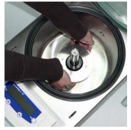
Abb. 57: Removing the rotor shaft
