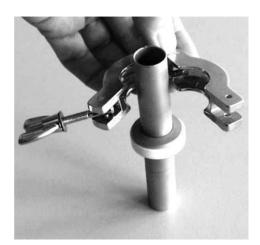
Fig. 53: Attaching the clamping ring
