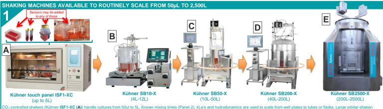
disposable bioreactors have working volumes of 4L-12L (SB10 – B),10L-50L (SB50 - C), 40L-200L (SB200 - D) and 200L-2500L (SB2500 - E) and also have well-known mixing times and kLa's. Orbital-shaken single-use bioreactors offer straight-forward process scale-up. Panel 3 shows mixing times, kLa's and OTR's for the SB10-X. CHO-K1 cultivation comparison to a 1L stirred bioreactor is shown in panel 4.
